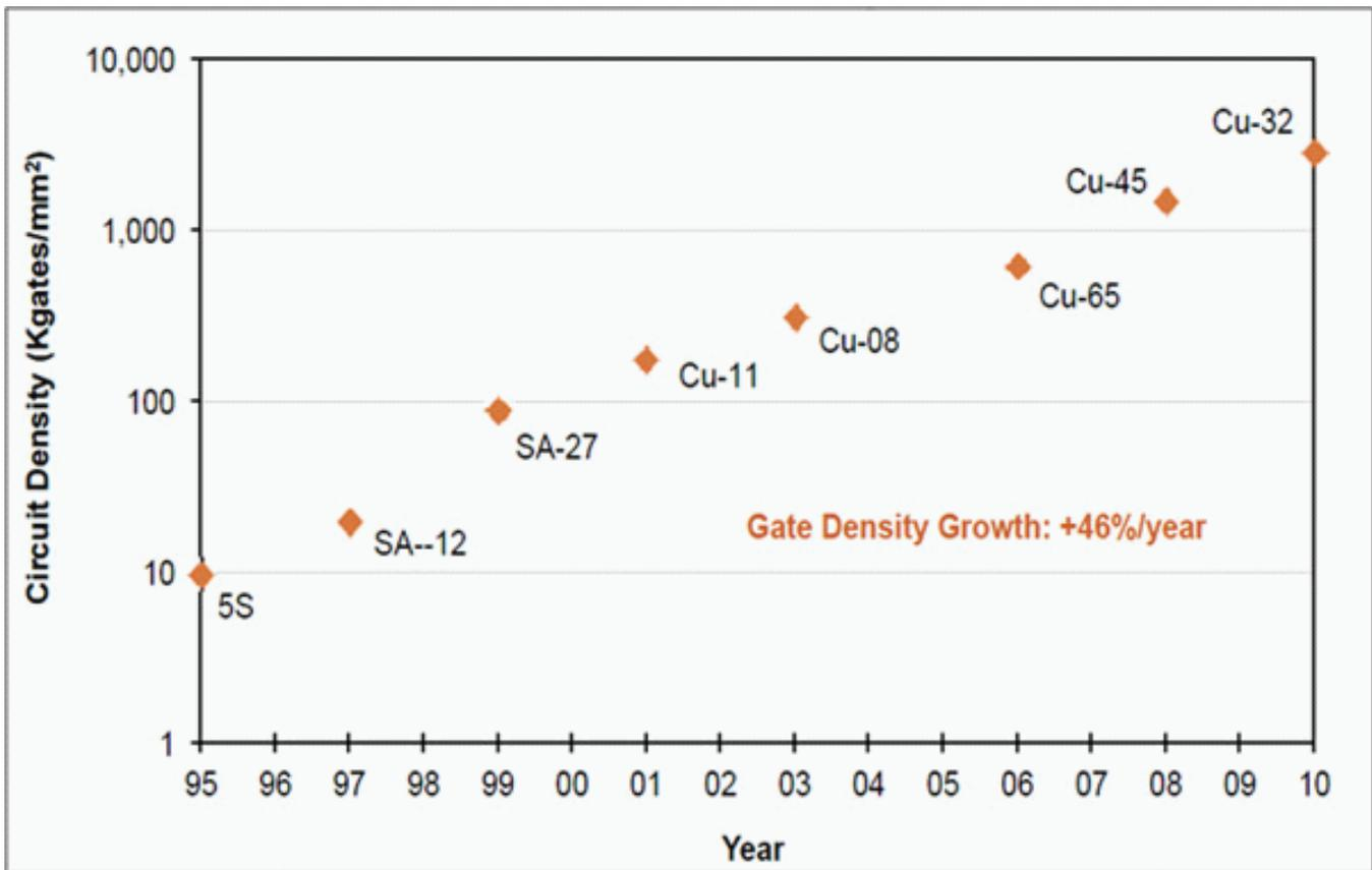
Fig 1. As an example of today's ASIC design complexity, IBM's Cu-32 ASIC product offering delivers 2.9K raw gates per square millimeter. Such advanced process nodes enable SoC design teams to integrate and implement extremely powerful and complex systems, and designers are taking advantage of these available gates. (Source: The McLean Report 2011)
